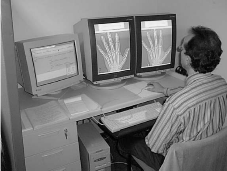
Figure 26 Image analysis workstation displaying digital images from serial examinations. Images are blinded to treatment and chronological order, edge-enhanced, and read in side-by-side comparison. This is combined with special measurement and reporting tools and automatic databasing of the results.
